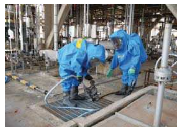
Chemical Attack team close valve on suction and discharge of HP – 212A and clear water contaminate ACH to HD - 260
